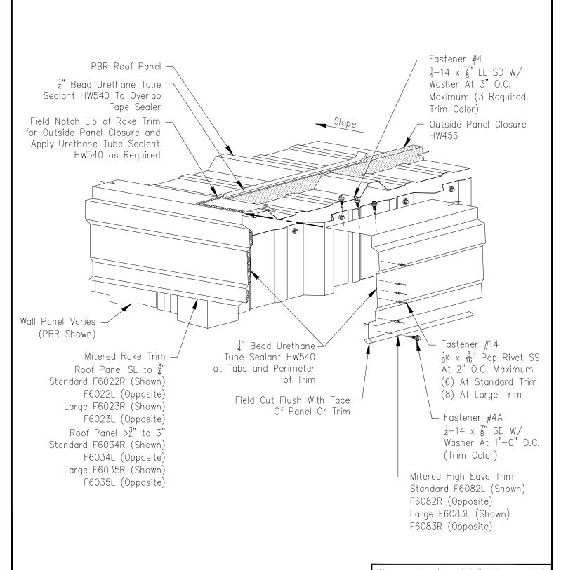
See construction details for required attachment of eave trim and rake trim to roof and wall.
